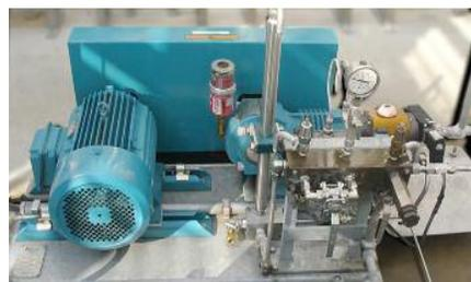
A reciprocating Cryogenic Pump used in a cylinder filling center
